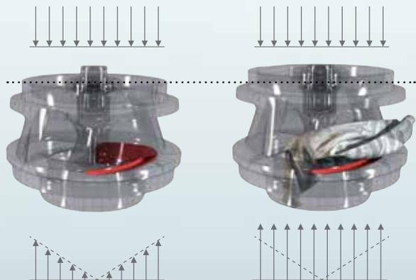
Fig 1: Hydraulic force distribution in normal operation
