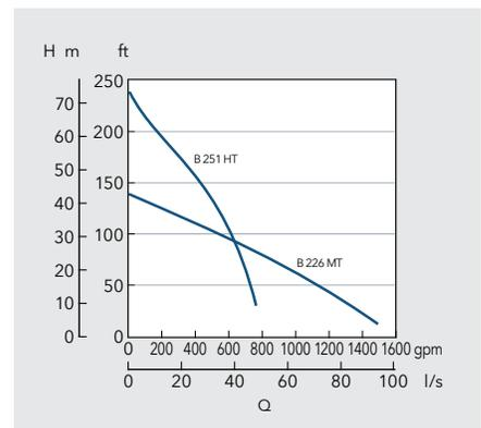
SH=Super high head HT=High head MT=Medium head B=Wear resistant impeller K=Open impeller
